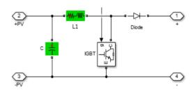
Figure 4. Boost Converter Topology
