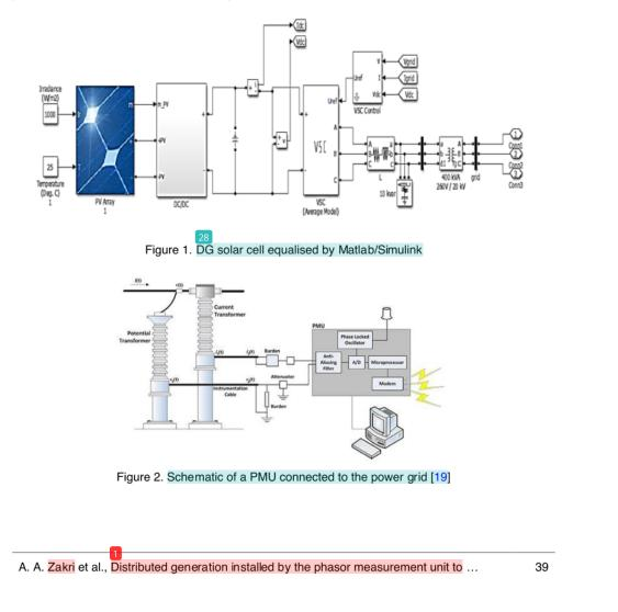
The MPPT P&O algorithm uses voltage and current, where the voltage and current detected is able to increase or decrease the duty-cycle the boost converter circuit is provided. Also, the threephase inverter used to supply dc voltage is obtained from a large capacitor connected to the input terminal to reduce the harmonic feedback
