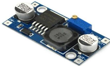
Gambar 2.9 Modul Step Down LM2596
