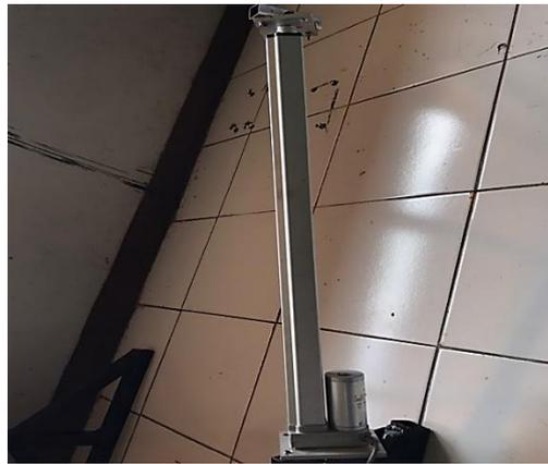
Gambar 3.4 Motor DC/Aktuator
