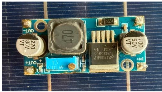
Gambar 3.8 Modul Step Dwon LM2596.
