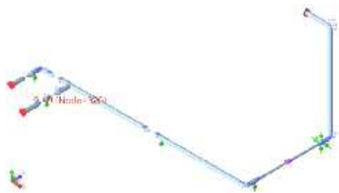
Fig. 10 Sustained load simulation result on CAESAR II
