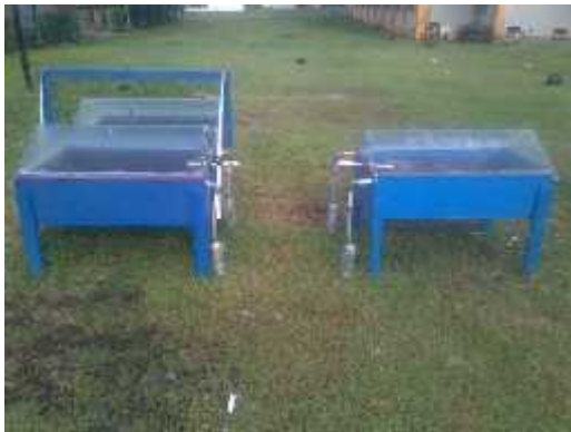
Figure 1. solar distillation to process sea water into freshwater and salt
