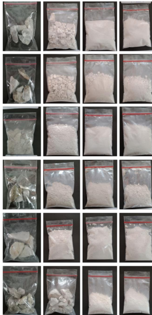
Figure 1. Different visualization of quicklime produced after calcination from different temperatures
