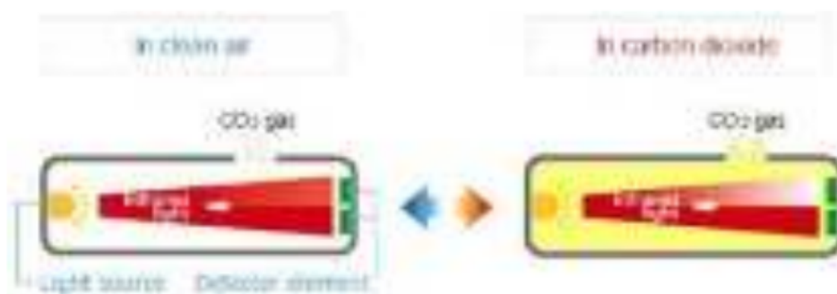
Gambar 3.7 Prinsip kerja sensor tipe NDIR [Figaro, 2021]
