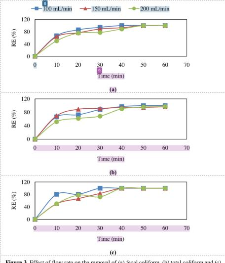
**Figure 3.** Effect of flow rate on the removal of (a) fecal coliform, (b) total coliform and (c) *Salmonella* after 60 minutes plasma treatment (RE: removal efficiency)
