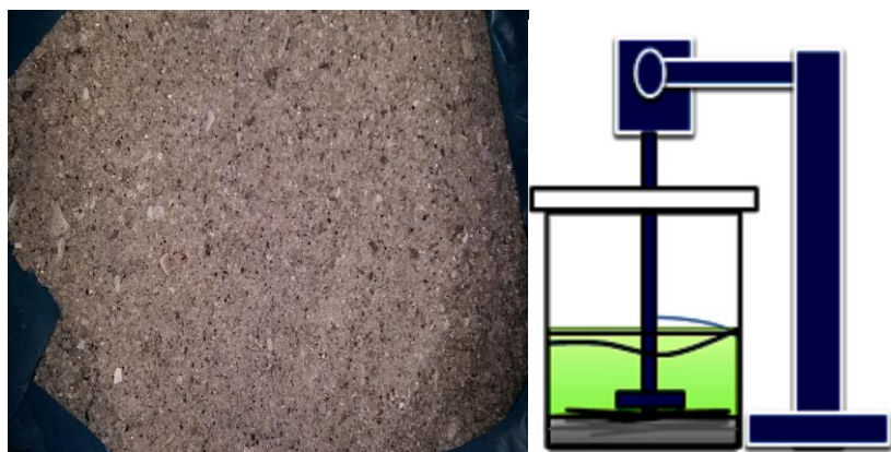
Figure 2.1 (A) White Sand and (B) Propeller in Cleansing the Sand
