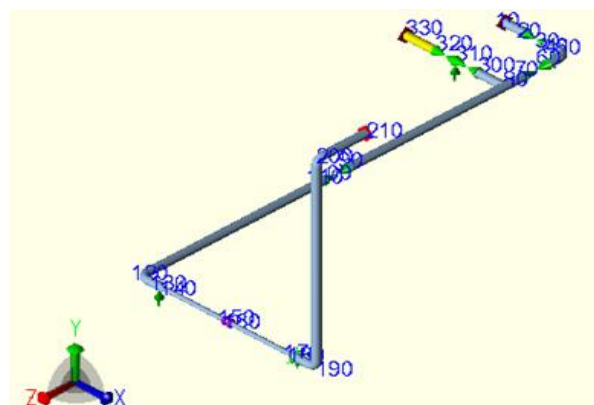
Fig. 6 Modelling shown from the results of data input in CAESAR II
