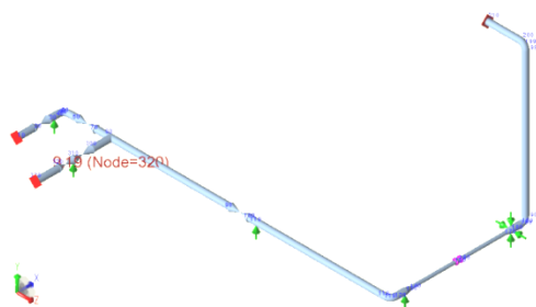
Fig. 10 Sustained load simulation result on CAESAR II
