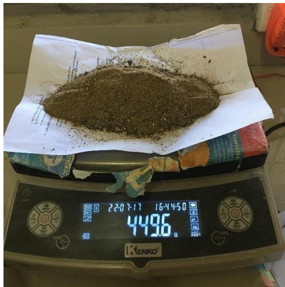
Penimbangan Berat Agregat Kering Oven Cuci
