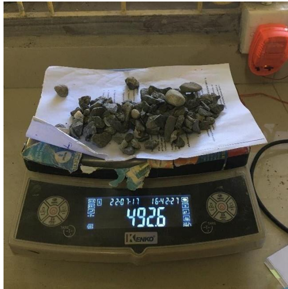
Penimbangan Berat Agregat Kasar Kering Oven Cuci
