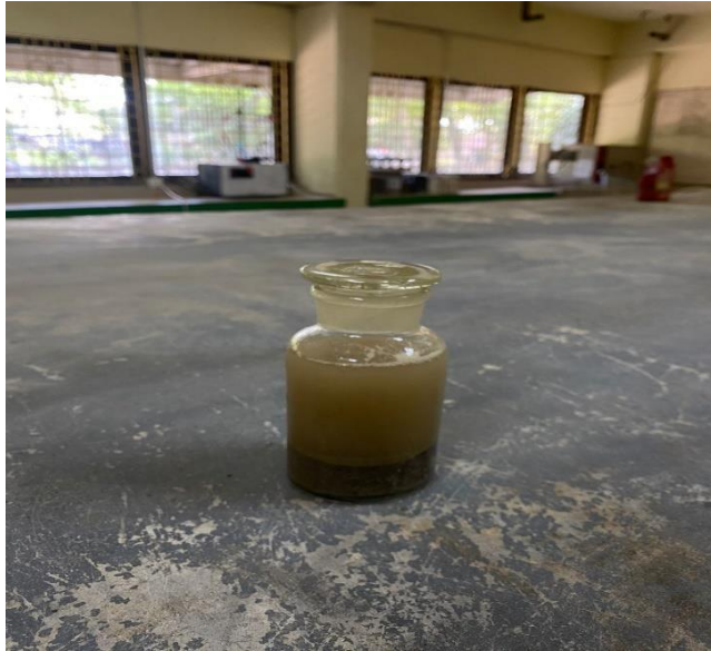
Hasil Pengujian Kadar Organik Abu batu
