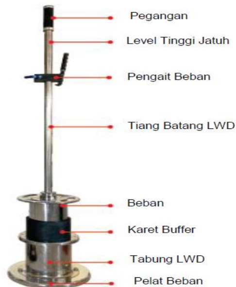
Gambar 2.1. Peralatan Light Weight Deflectometre (LWD)
