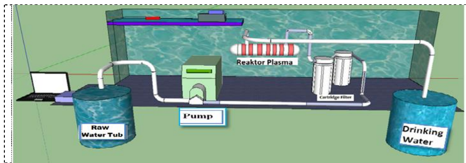
Figure 1. Experimental set-up of radio frequency plasma-filtration system
