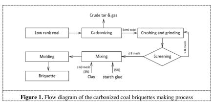
The composition of the briquette mixture consisted of charcoal 92%, filler 3%, and binder 5%. The use of filler intended to absorb gas emissions and to reduce the fly ash phenomenon during the cooking process. Meanwhile, the use of binder is intended to provide strength to the briquettes so that they are not easily destroyed during transportation, storage, and use[5]. The last step of the briquette making process was the briquettes molding, which was conducted manually.
