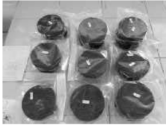
Figure 2. Biobriquettes of Mixture of Biomass and Adhesives
