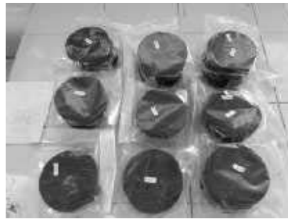
Figure 2. Biobriquettes of Mixture of Biomass and Adhesives
