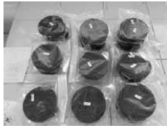
Figure 2. Biobriquettes of Mixture of Biomass and Adhesives
