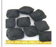
**Figure 4.** Typical jengkol briquette
