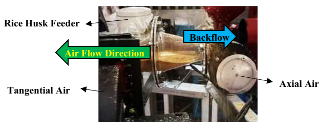
Fig. 6 Backflow phenomenon in the cold test experiment
