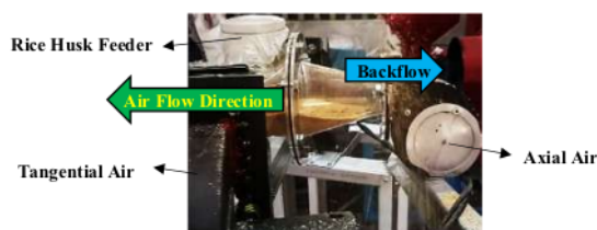
Fig. 6 Backflow phenomenon in the cold test experiment
