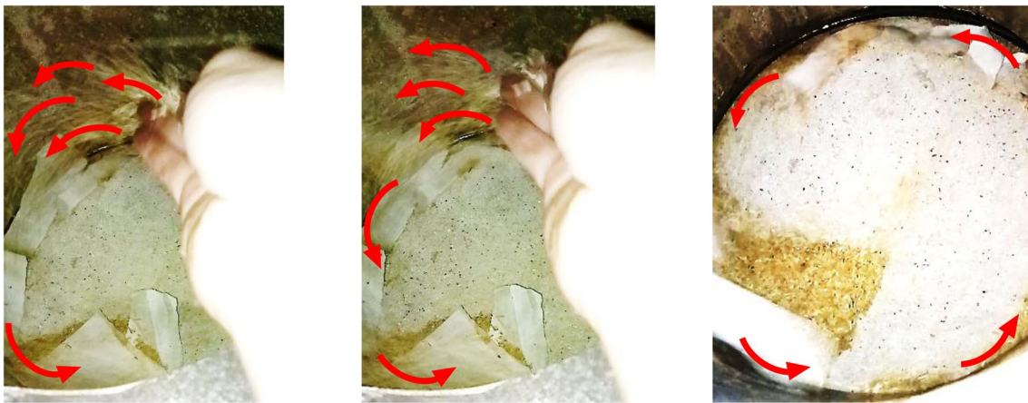
Fig. 5 Air and rice husk swirl flow pattern at the bottom area of suspension furnace (Red arrow indicates flow direction of rice husk)
