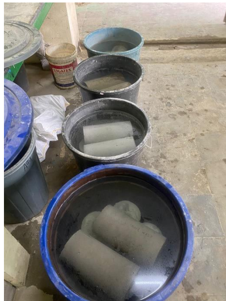
Proses Curing Beton
