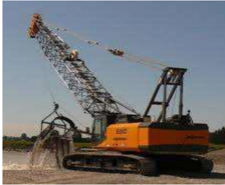
Gambar 2. 3 Crane Spun Pile
