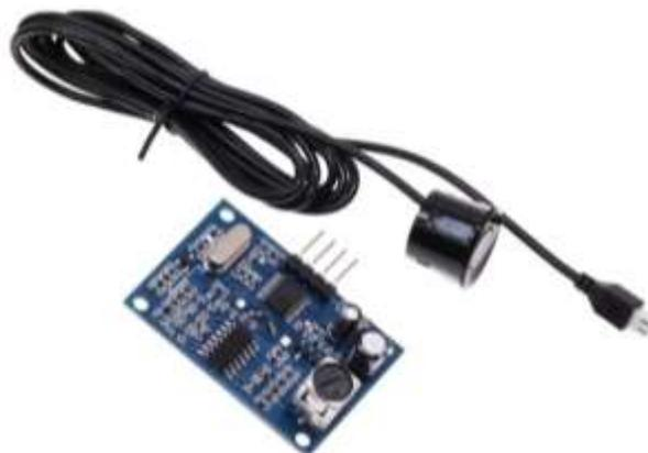
Gambar 3.7 Sensor Ultrasonik tipe JSN-SR04T
