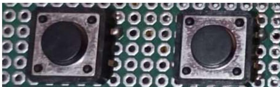
Gambar 3.10 Mini Push Button Switch
