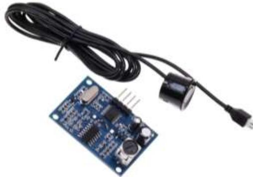
Gambar 2.5 Sensor Ultrasonik JSN-SR04T
