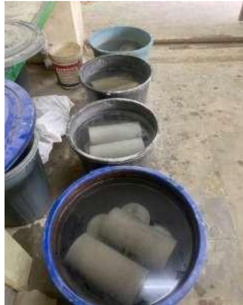
Proses curing beton
