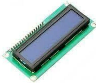
Gambar 2.5. *Liquid Crystal Display (LCD)*
