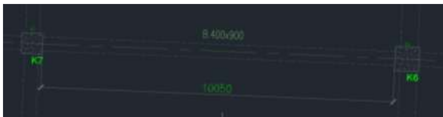
Gambar 3.2 Bentangan Balok AS T1.1/T1.C
