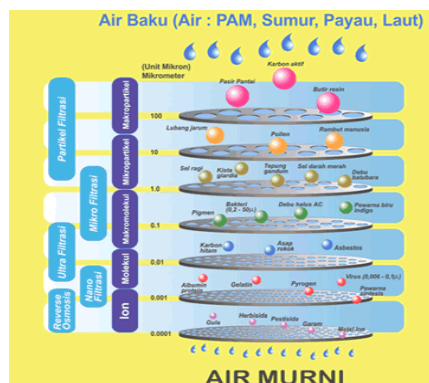
Gambar 5.4 Proses pengolahan Reverse Osmosis
