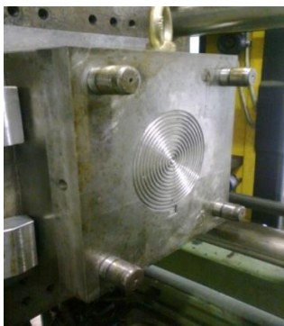
Fig 1. a) Spiral mold and b) Resulting samples, generated from a variety of compositions
