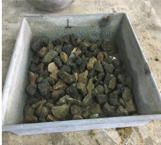
**Gambar 3.9 Proses Perendaman Agregat Kasar**
