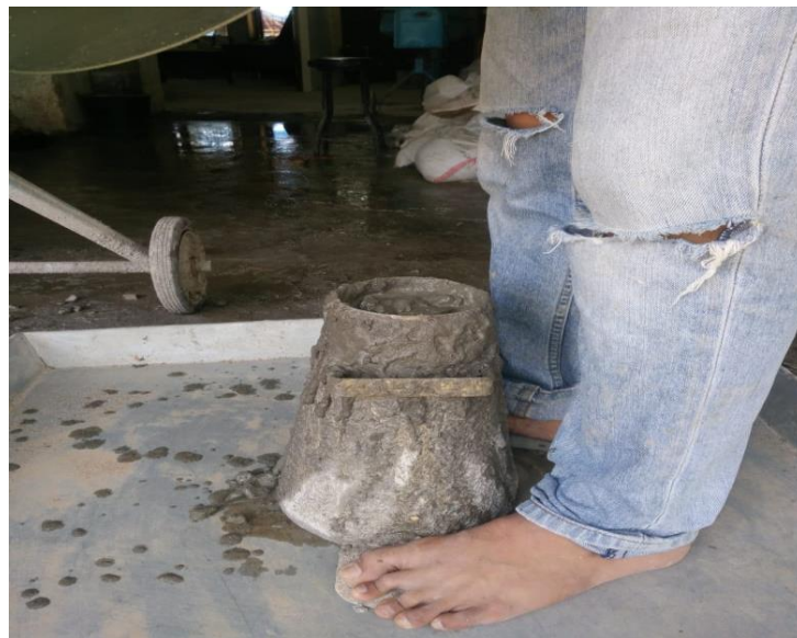
Lampiran.24 Proses pengujian slump flow
