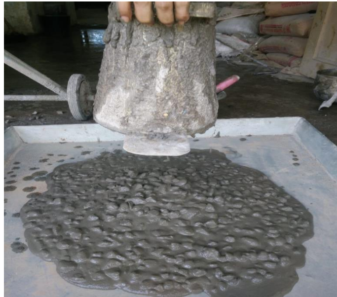
Lampiran.25 Proses peengujian slump flow
