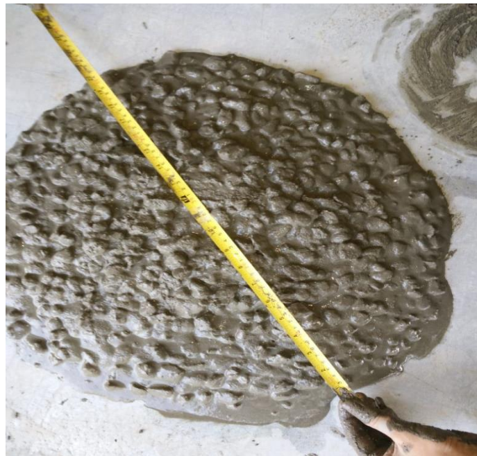
Lampiran.26 Pengukuran slump flow
