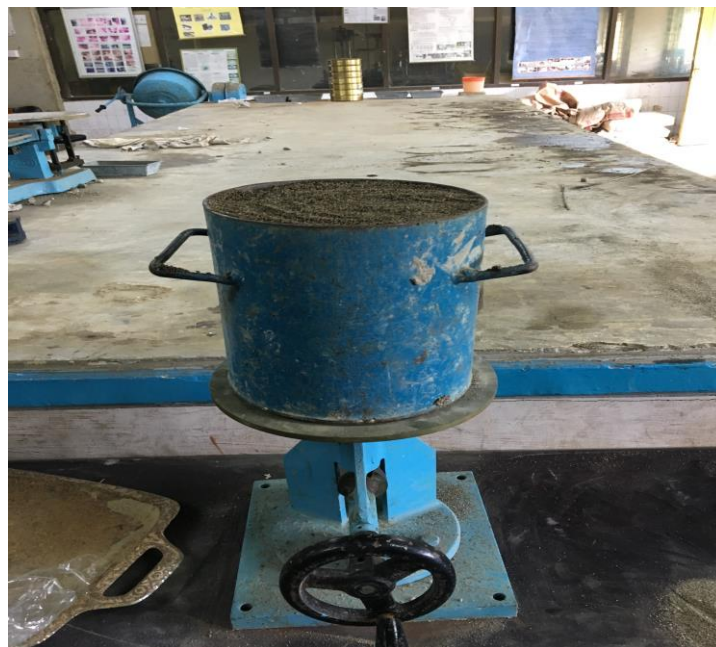
Lampiran.8 Proses pengujian bobot isi
