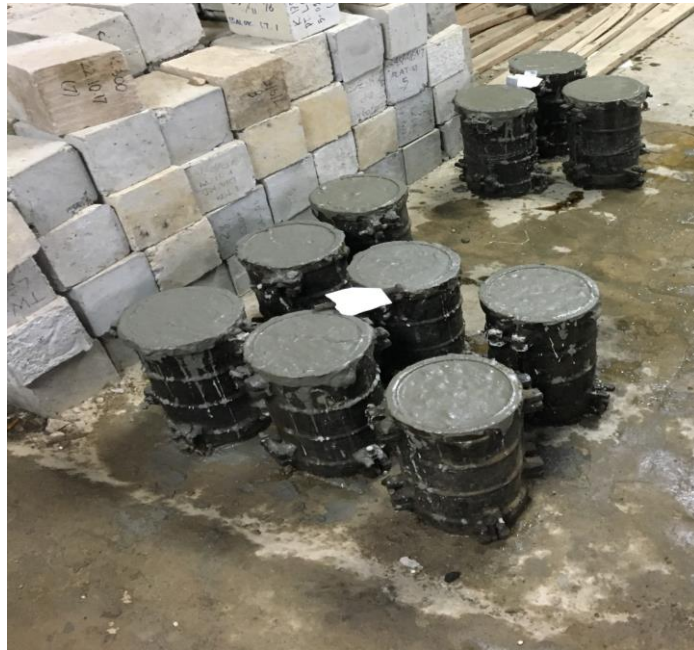
Lampiran.31 Proses pengeringan sample beton
