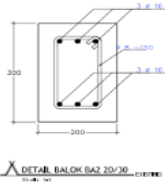
Gambar 41. Pendetailan Balok BA (20/30)
