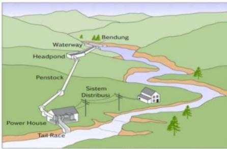
Figure 1. General Schema and RORMPP Components [4]
