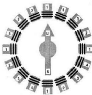
**Gambar 2.22** Skema motor stepper
