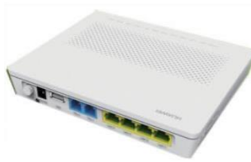
Gambar 2.35 Optical Network Terminal
